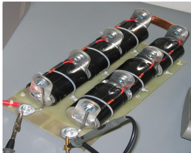
Fig. 8 The supercapacitor battery consisting of 6 devices with 600F capacity coupled in series with a total rated voltage of 12 V
