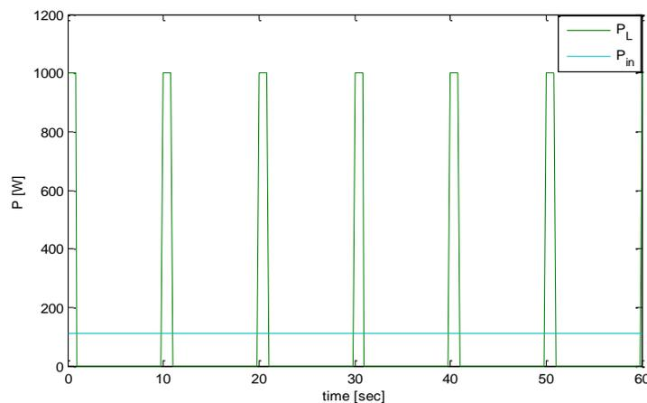
Figure 10 – constant power charging and pulse discharging
