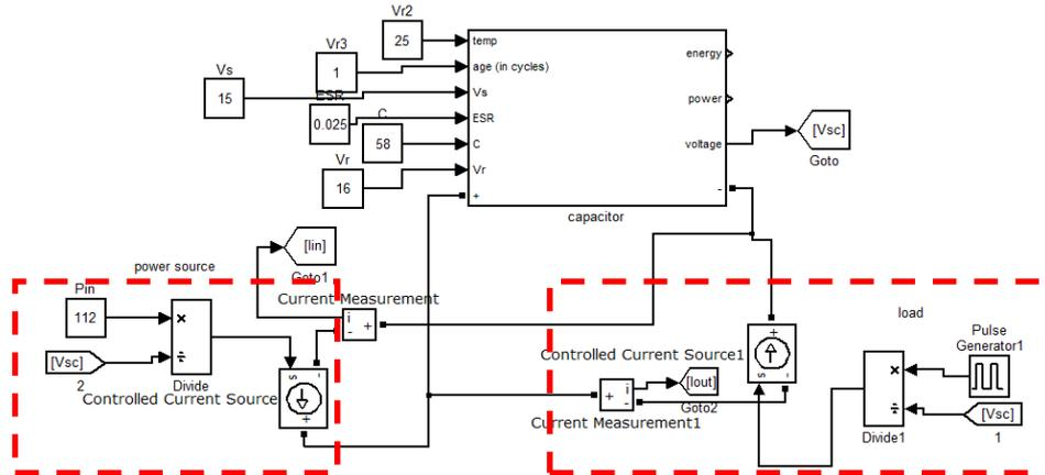
Figure 9 – simulation description of charging station
