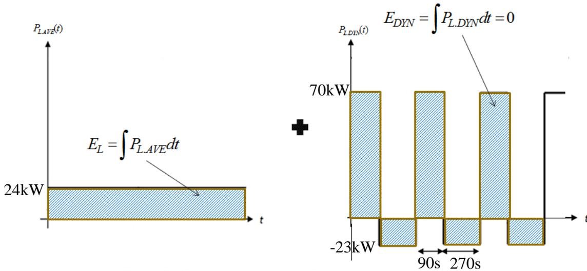
Figure 8 - Splitting the power profile into average and dynamic parts
