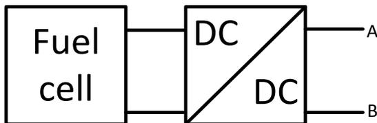
Figure 5 – Bufferless topology
