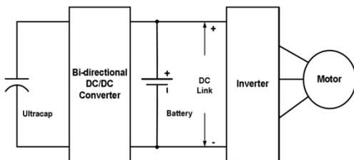
Fig. 4: Ultracapacitor/Battery active configuration[2]
