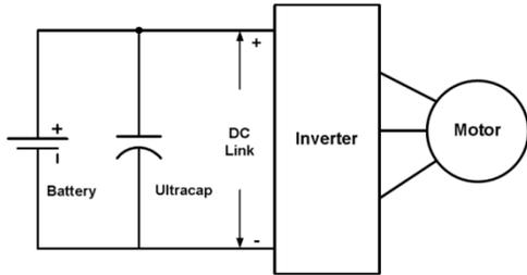
Fig.2: Passive parallel configuration[2]
