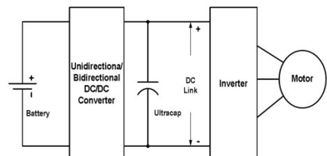
Fig. 5: Battery / ultracapacitor active configuration[2]
