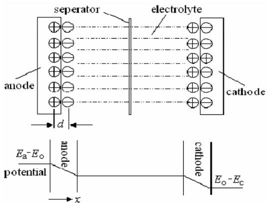
Fig 7: Schematic of super capacitors and potential Distribution throughout electrochemical capacitor During charge
