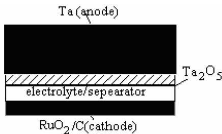
Fig. 9: the structure of hybrid capacitor[6]
