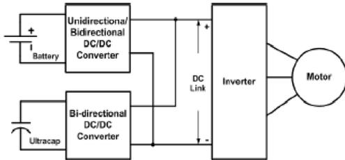
Fig. 6: Multiple converter active configuration[2]
