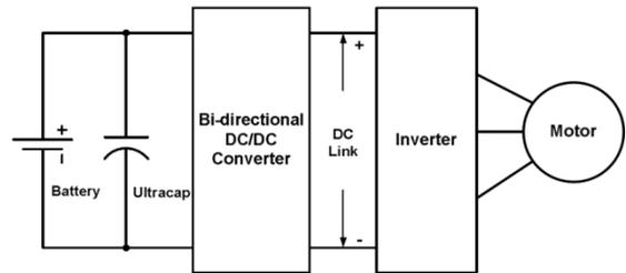
Fig.3: Passive parallel with bidirection DC/DC converter[2]
