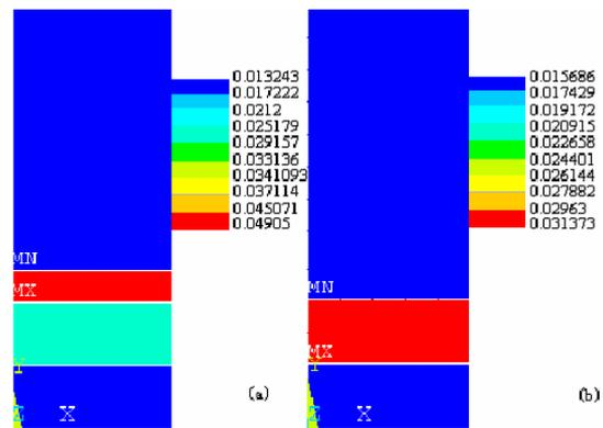
Fig. 10: The electrostatic field of hybrid capacitor: (a) It has Ta2O5 membrane (b) with no Ta2O5 membrane [6]
