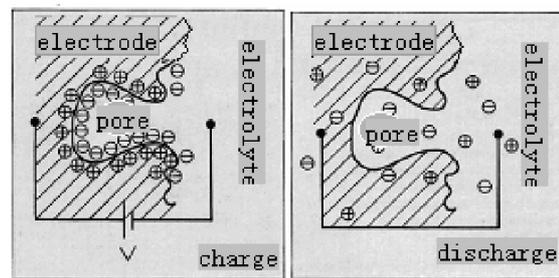
Fig 8: The structure of double layer charge during charge and discharge
