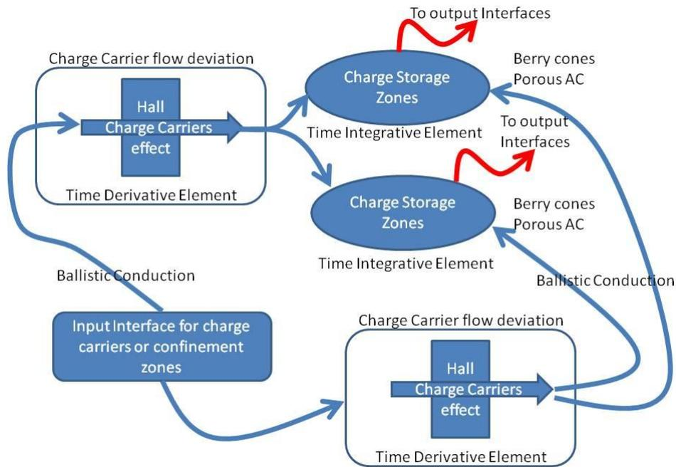
Fig 1 Path oriented walking architecture: Input interfaces or confinement zones; walking paths based on ballistic conduction on 2D graphene; sensing and eventually threshold elements; charge carriers collector zones with or without sensing and eventually threshold elements. All these elements can be placed on a single or adjacent multiple graphene or other condensed matter layers
