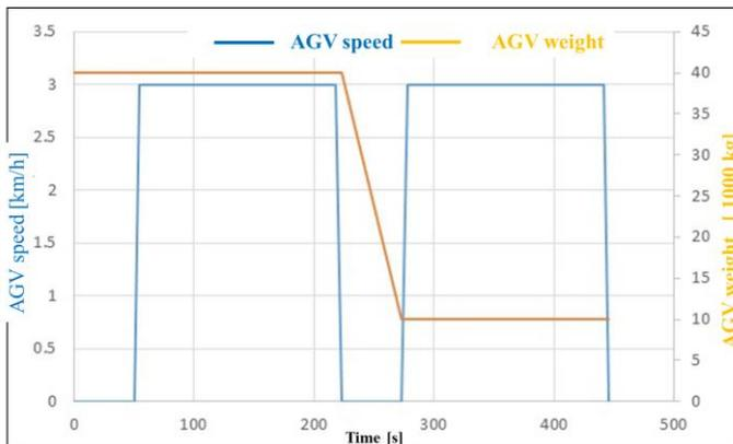
Fig. 2. AGV average duty cycle.
