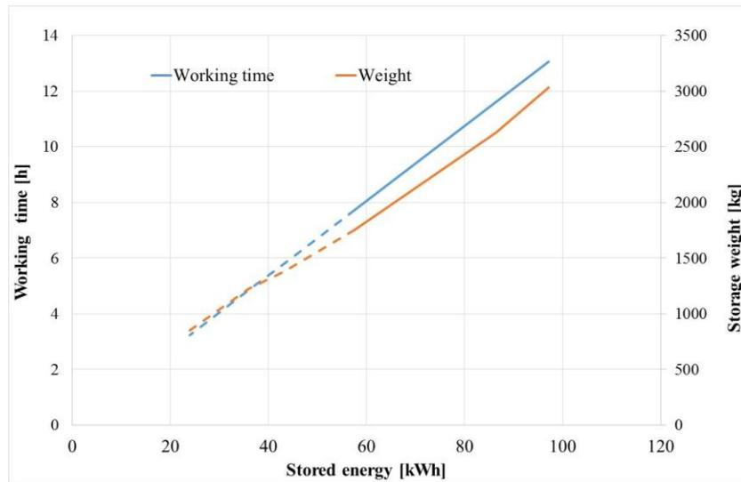
Fig. 5. The variation of working time of the AGV and weight of the lead-acid battery as a function of the available energy on board.
