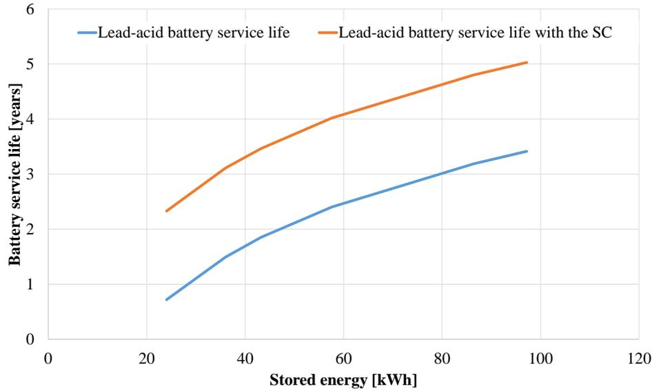
Fig. 6. Service life of the lead-acid battery with and without the SC bank.
