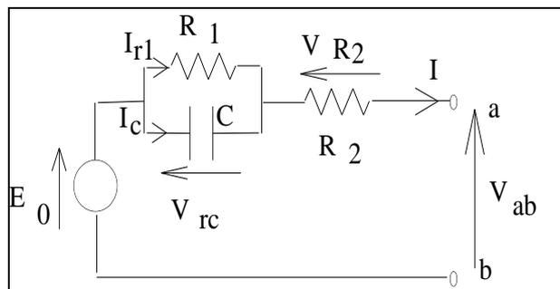
Fig. 4. The equivalent electric circuit of a lead-acid battery.
