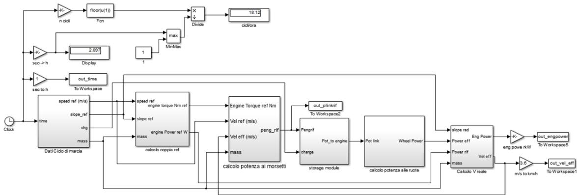
Fig. 3. The simulation model of electric vehicles, used at ENEA.
