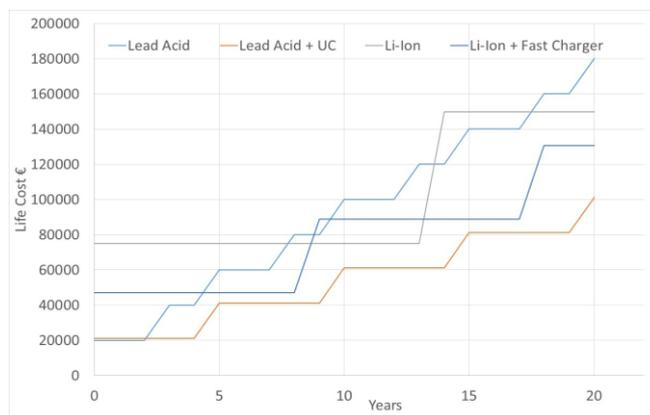
Fig. 9. Economic comparison of the various storage solutions for the AGV case.
