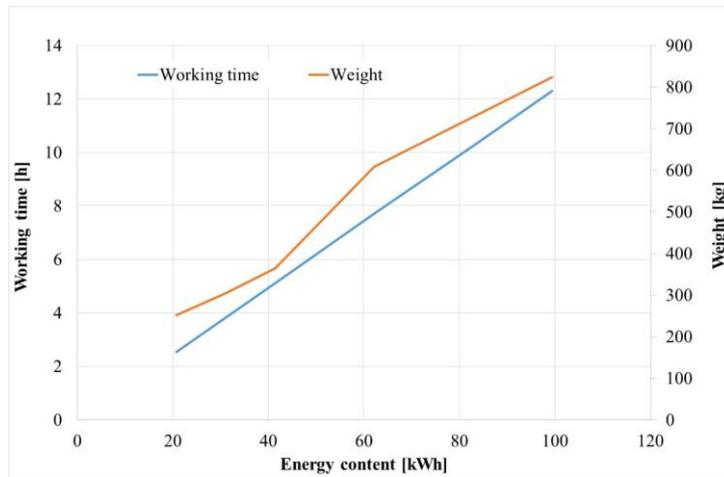
Fig. 7. Li-ion service life and weight in function of the energy content.
