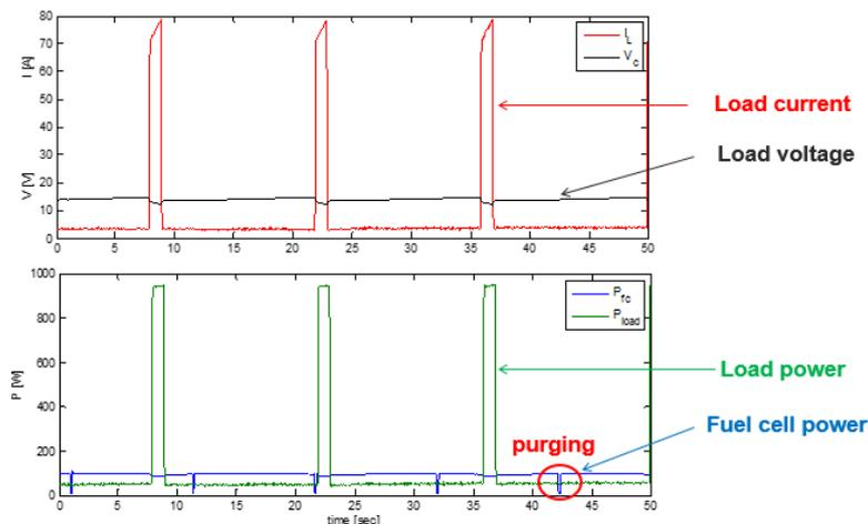
Figure 1: Sample experimental results. Top: load current and voltage; Bottom: load and fuel cell powers
