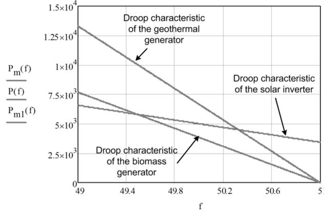
Fig. 3. Droop characteristic of the generators and the inverter.
