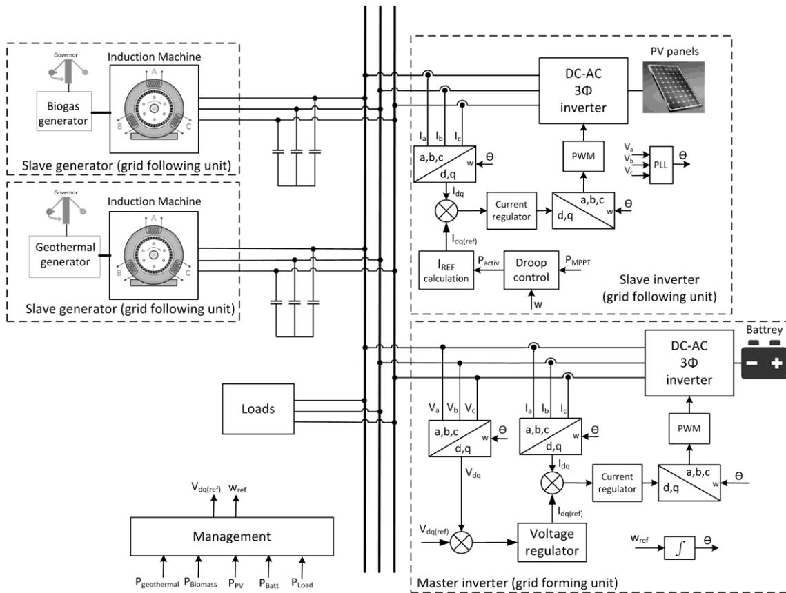
Fig. 2. Microgrid proposed control concept.
