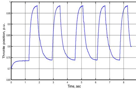
**Fig.11: Throttle control due to Look-up-table algorithm**
