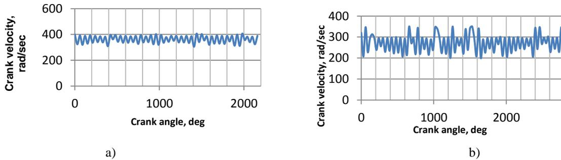
**Fig.6:** Changing of crank velocity versus angle of crank rotation: a) Full Throttle (FT), 0A current; b) 30% of FT, 20A current.
