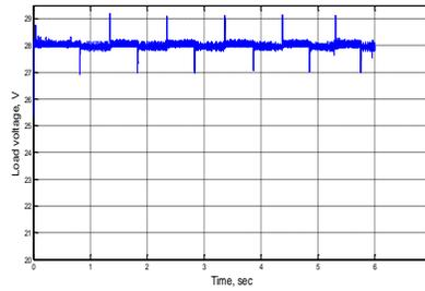
**Fig.14:** Output voltage deviations during ACTR
