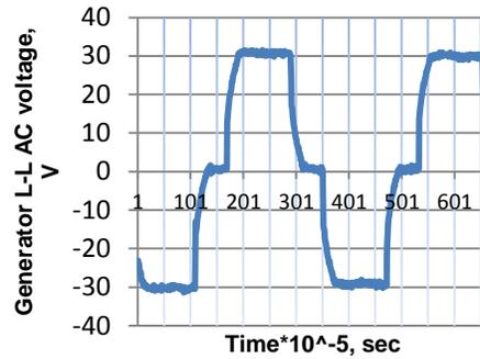
**Fig.5:** A sample of AC Line-to-Line voltage before a rectifier
