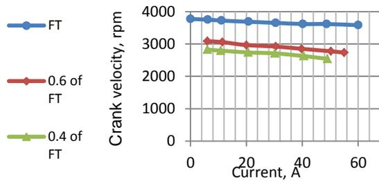
**Fig.7:** Crank velocity drop versus increasing load current for different throttle positions
