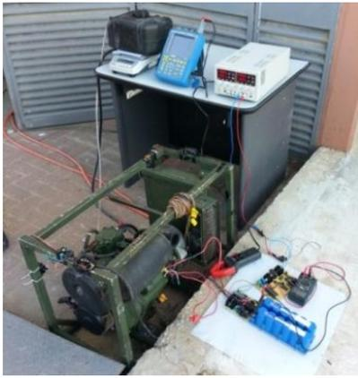
**Fig.1:** Experimental set-up for testing diesel generator Yanmar L48AE.
