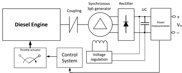
**Fig.4:** Diesel generator with the system of throttle position control.
