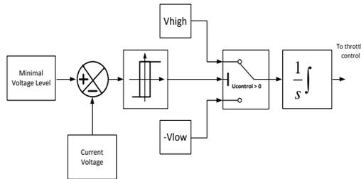
**Fig.9: Principle block-diagram of ACTR control**
