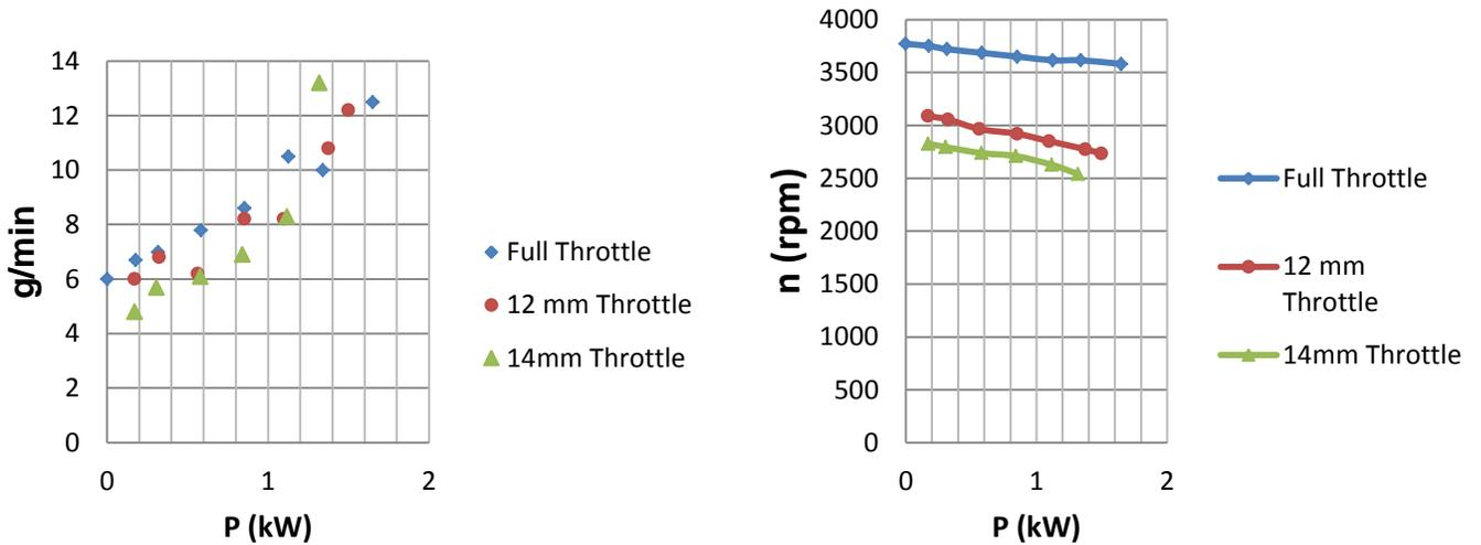
**Fig.3:** Experimental results of fuel consumption and rotation velocity for different throttle positions.
