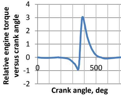
**Fig.8: Engine torque produced during rotating crank angle**
