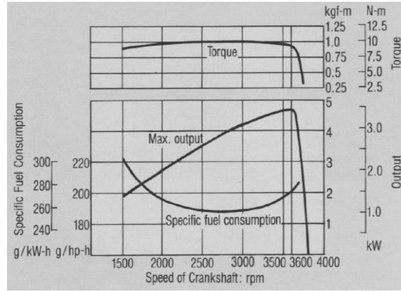
**Fig.2:** Typical output curves diesel generator Yanmar L48AE.
