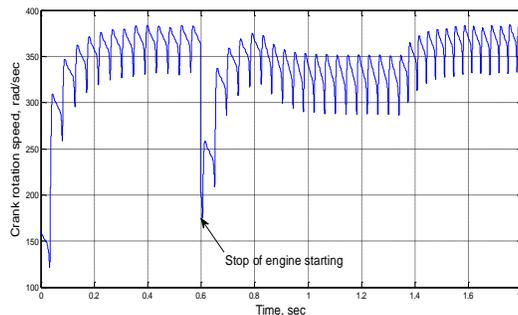
**Fig.15:** Crank (generator) rotating velocity during the time
