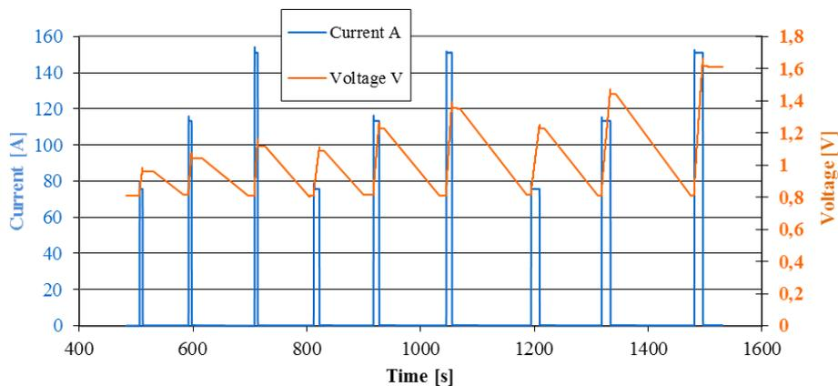
Fig. 4. Fast charge test profile for BCAP3000 cell.
