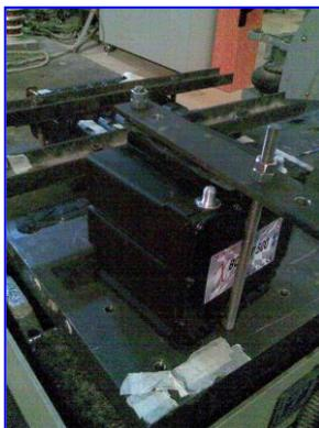
Fig. 11. The SC module on the electrodynamic shaker.
