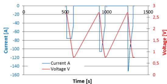
Fig. 5. Current and voltage profiles for peak power test.
