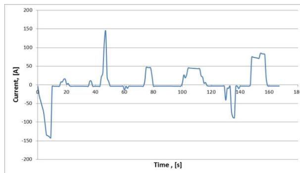
Fig. 7. ALTRA-IVECO current profile (micro-cycle) scaled down at cell level.
