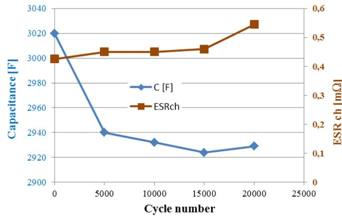
Fig. 8. Capacitance and ESR<sub>ch</sub> trends during cycle life testing.
