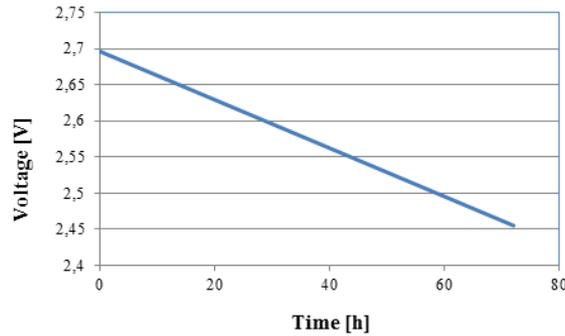
Fig. 6. OCV decline during self-discharge test.
