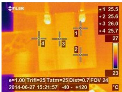
Fig. 11. Thermogram with an infrared camera of the SC module during life testing.
