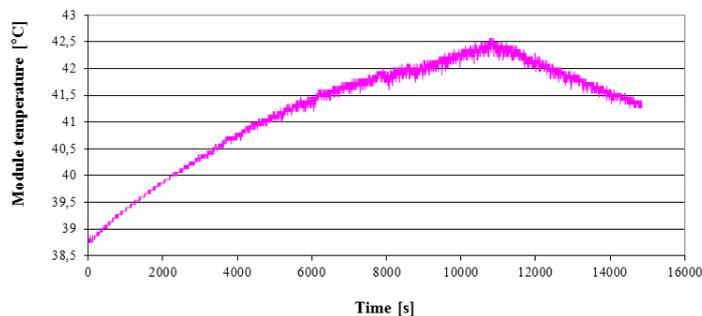
Fig. 10. Temperature variation during module testing with a test interruption after three hours.
