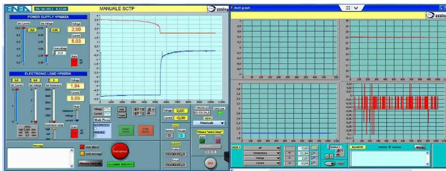
Fig. 3. User interface of the Labview SW during manual SC testing.
