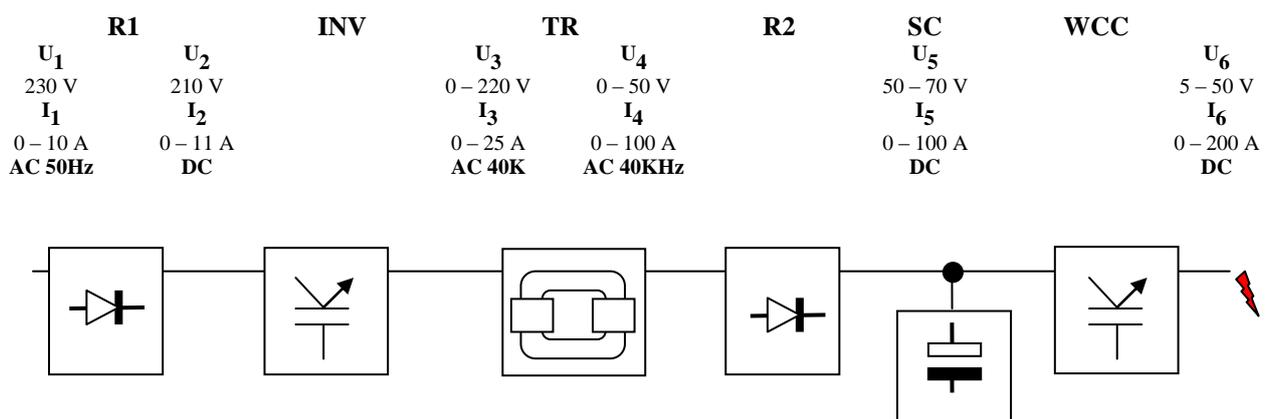
Figure 1 Structure of the power conversion chain with SC for the arc-welding supply
